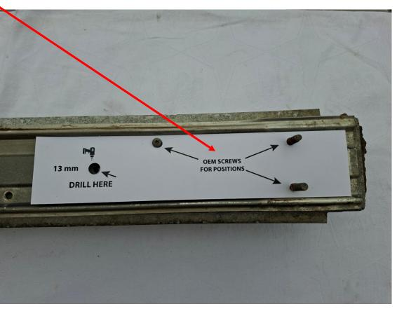
7. Drill completely through the aluminum structure and energy-absorbing foam at the points marked on the drilling template using a size 13 drill bit.
