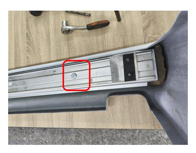
12. Screw the bumper onto the factory mounting structure.
