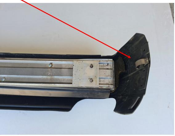
3. Screw the thin aluminum plate back on.
